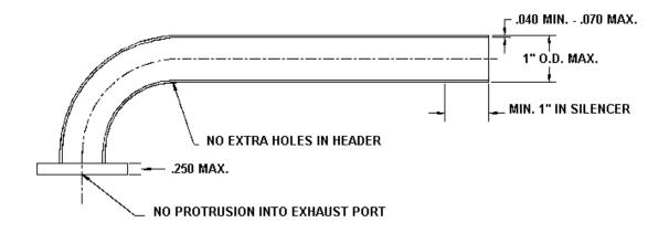
NOTE: A header that is broken, kinked or cracked in the tubing may be replaced at any time during the event under the supervision of a Technical Official. A header damaged during the event may pass post race inspection and the competitor will not be penalized, assuming the broken header/silencer remains attached to the kart (safety wire, bracket, etc). Any header/silencer not attached to the kart cannot be inspected by a technical official, resulting in exclusion from the event.
